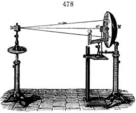
upon the bulb of the thermoscope, placed at the point where the rays are brought to a focus. The temperature indicated by the thermoscope is found to vary with the nature of the plates.
