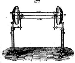
conveyed to the focus B, igniting the gunpowder or phosphorus placed at that point.
